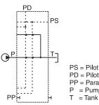
PS = Pilot Supply PD = Pilot Drain PP = Parallel Path = Pump
